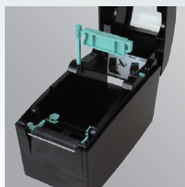
Enhanced label feeding mechanism
